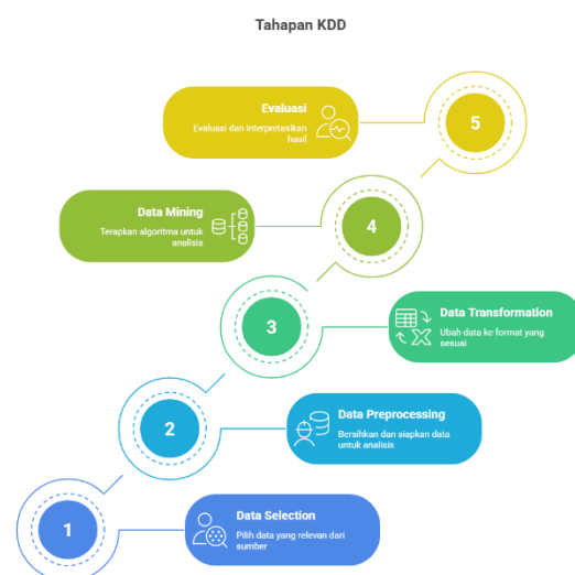
Gambar 1. Tahapan Knowledge Discovery in Database (KDD)
